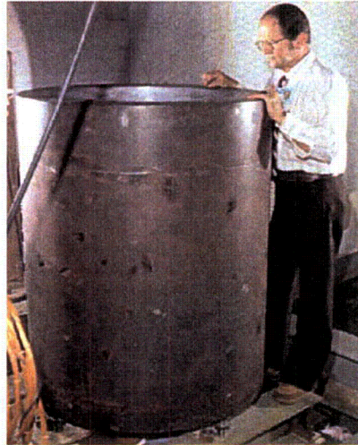
Fig. A-3.4. TSE test cylinder like those used in TSE-5, -5A, -6, and -7.
