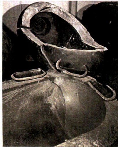
Fig. A-2.3. ITV-2 vessel was tested under high pressure and at a temperature (32°F) low in the Charpy transition region; fracture was by fast cleavage propagation.
