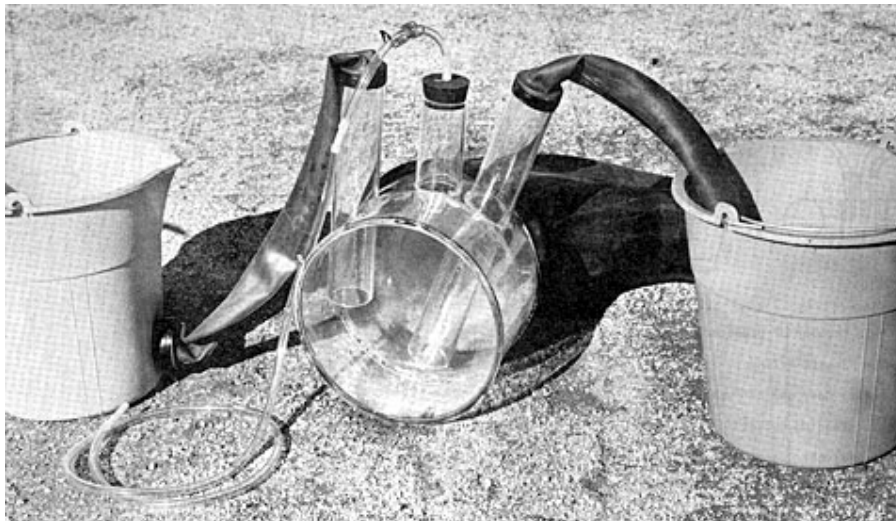
Fig. 21 Attachment of pipes and buckets
