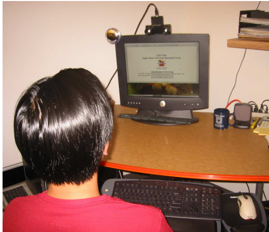
Figure 9: Experimental setup. A stereo camera is placed on top of the screen to track the head position and orientation.
