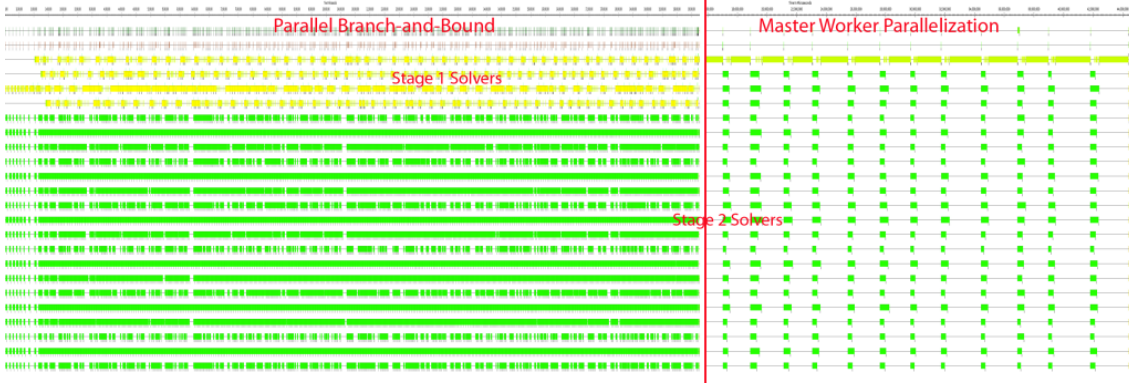
Figure 5.1: Projections traces compare processor utilization of the branch-and-bound and master-worker implementations (Chapter 3). Thick colored bars of each horizontal trace represent individual processor activity across time; thin gray lines indicate idle processors. The figure shows that processors are used more efficiently in the parallel branch-and-bound schema.
