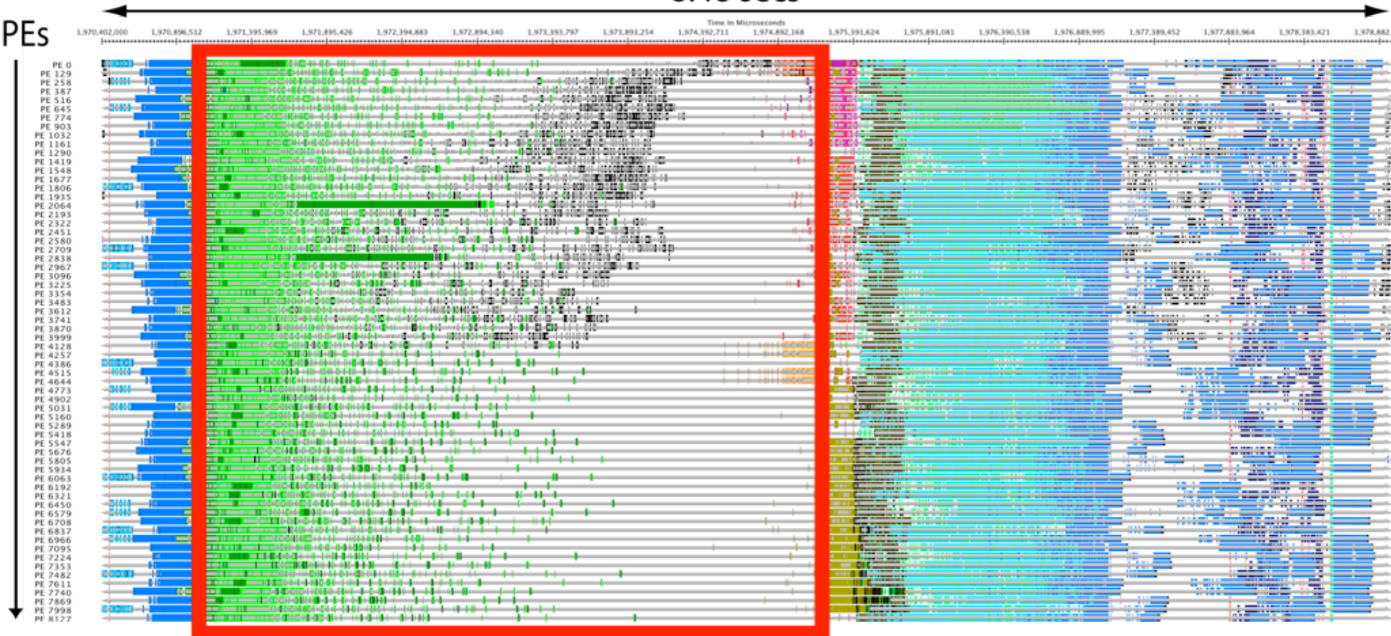
Timeline view (OpenAtom on 8,192 cores of BG/L) using the performance visualization tool, Projections
