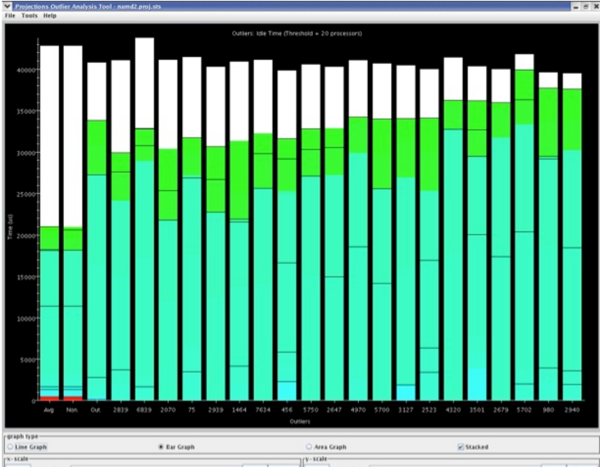
Figure 3.15: The Extrema Tool presenting the top list of least idle processors.
