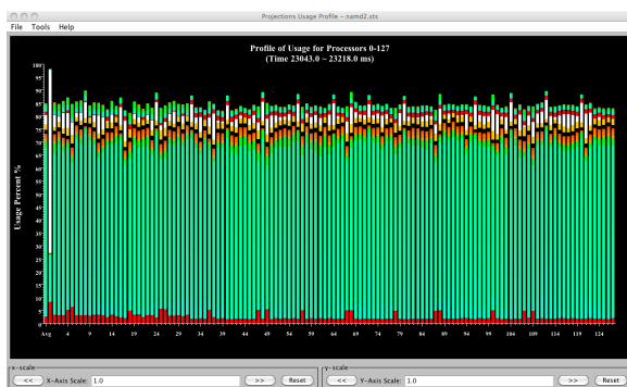
Figure 2.7: Usage Profile : Processor utilization of various activities.
