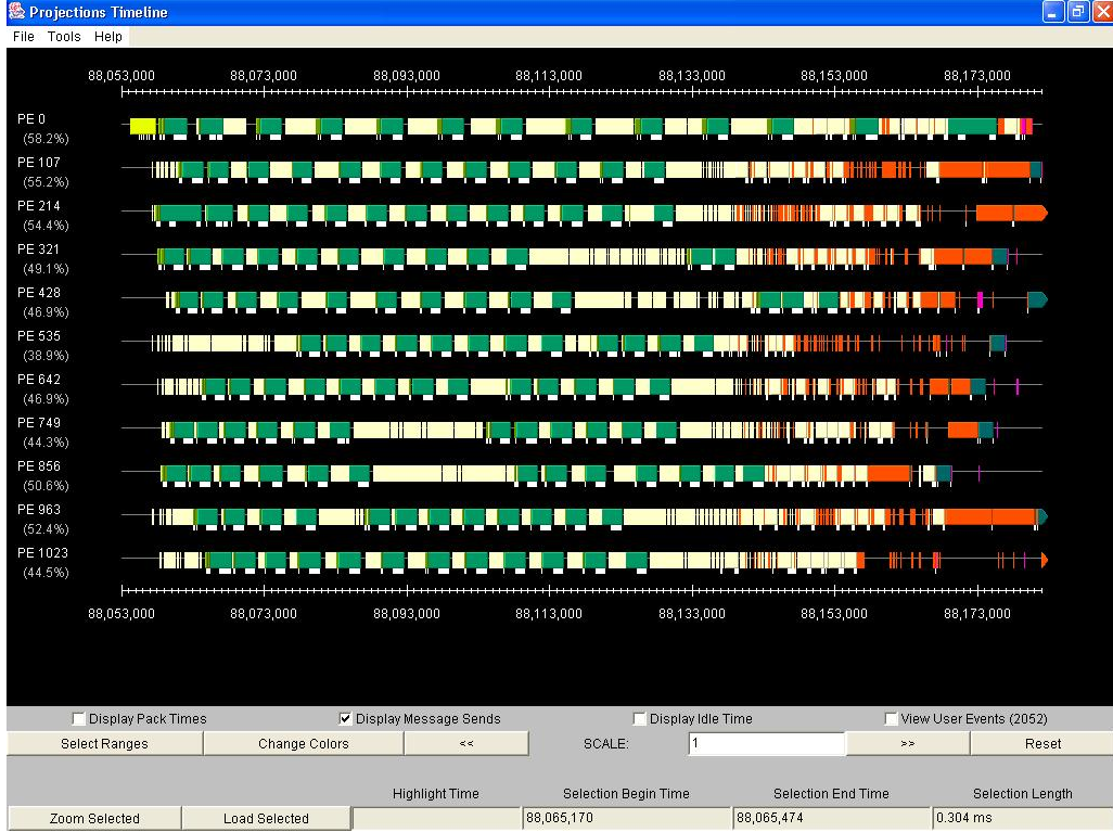
Figure 2.8: Overlapped Transposes in concurrent FFTs in Phase I, as seen in a timeline view. The x axis shows the time, and the y axis shows messages being processed on a subset of the processors. Some messages (show with tails) create new messages, the communication of which is overlapped with processing of other messages
