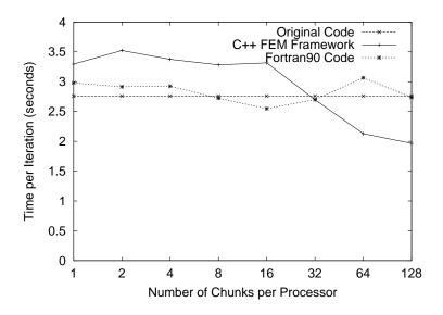
Figure 2: Effects of partitioning the mesh into chunks more than number of processors.
