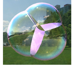
Figure 5: A triple-bubble at equilibrium exhibits a stable central Plateau border.
