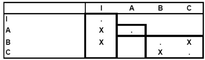
Figure 3: DSM for a modular design obtained by splitting.
