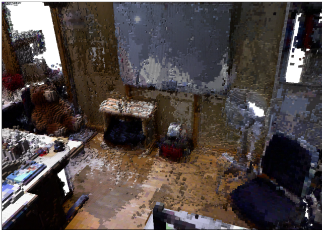
Fig. 5 Detail of a volumetric indoor OctoMap containing color information. The complete map covers an area of 7.3 \text{ m} \times 7.9 \text{ m} \times 4.6 \text{ m} at 2 cm resolution.
