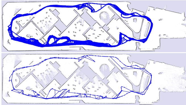
Fig. 1: The goal of our work is to prune the SLAM pose graph (top), maintaining a sparse pose graph (bottom), while minimizing the loss of information in the graph and the resulting map.
