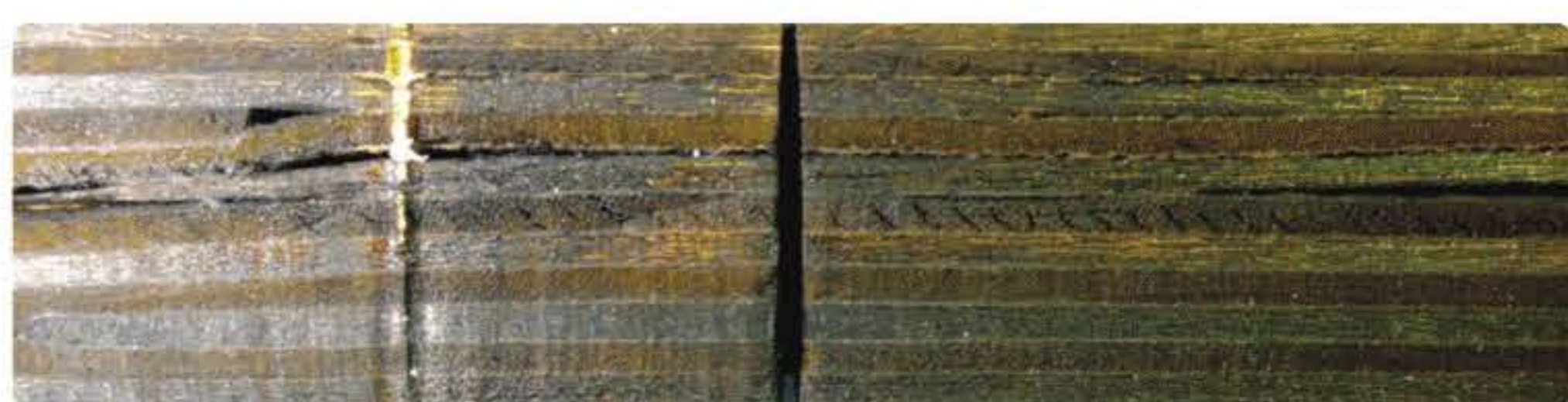
Kerf Verticality and Width Comparison
