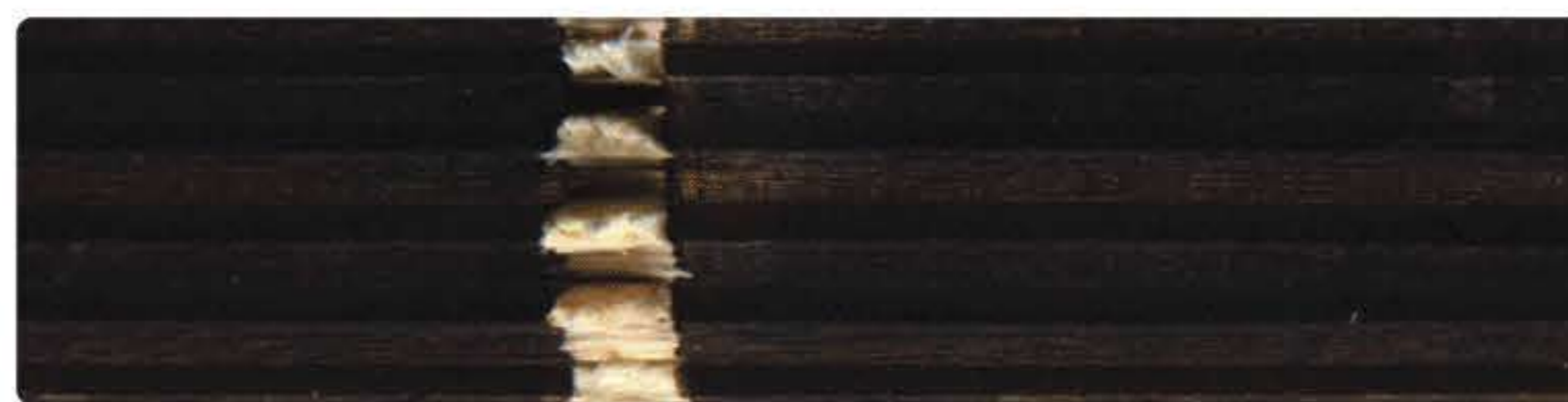
Wooden Fiber Kerf Surface and Carbonized Kerf Surface Comparison
