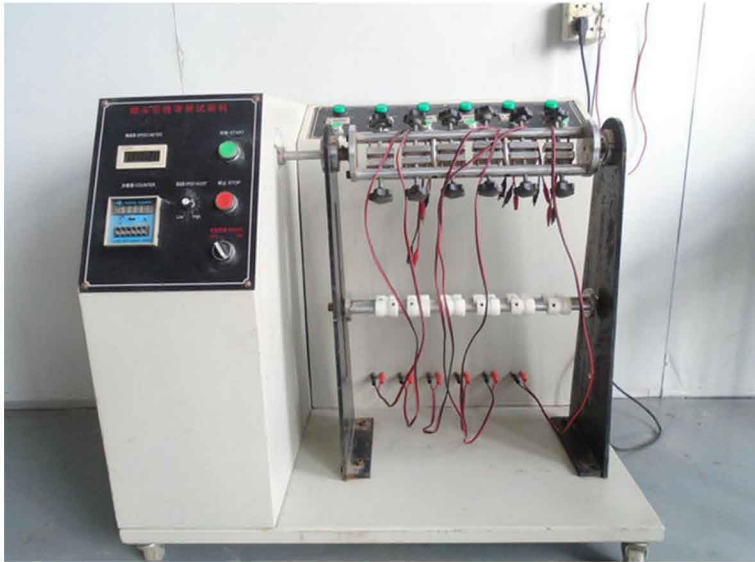
Resistance to bending test
