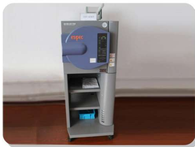
HAST高压低失重测试仪 HAST high pressure and low weight loss tester
