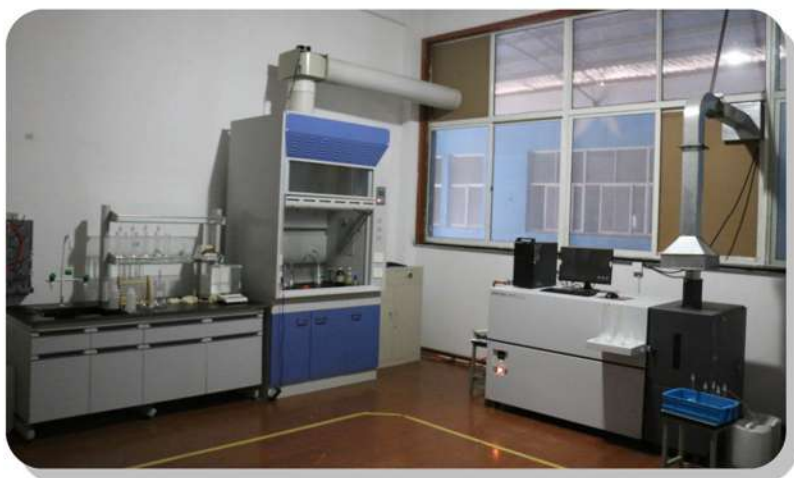
岛津ICPS稀土含量光谱仪 SHIMADZU ICPS content of rare earth spectroscopy
