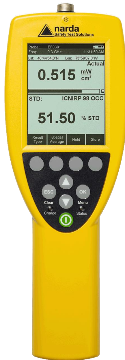
Narda Broadband Field Meter NBM-550
