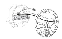
Connect the Neutral and Line wires (recommended strip length: 10-15 mm [0.4-0.6 in.]) to the silicone holes in the bracket. Secure the wires with a slotted screwdriver.
