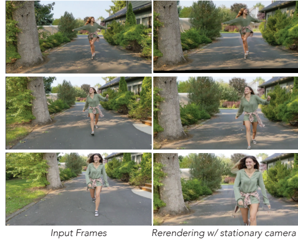
Figure 6. Camera stabilization. Our LDI representation can be re-rendered from new camera positions to produce stabilized or modified camera paths. Left: input video with camera dolly motion. Right: frames re-rendered from a stationary camera.
