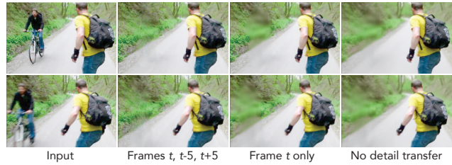
Figure 10. Detail Transfer Ablation. The background depth map allows reprojecting detail from nearby frames in time to further improve the visual quality of the predicted layers. From left to right: input frame, full result with detail transferred from frames t, t - 5, t + 5 , ablated result with detail only from frame t (note blurry region under bicyclist), no background detail transfer.
