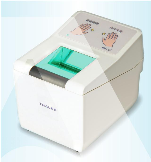
The Cogent Dual Finger Scanner DactyScan40i is a compact FBI certified fingerprint scanner integrating a 12 3-color led based graphical user interface to facilitate the acquisition process. It can be used in a wide range of applications where dual, rolled and flat fingerprint acquisition is required:
