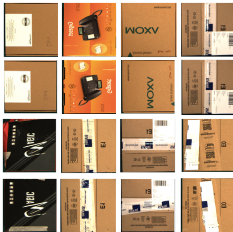
Fig. 9 Comparisons between warped images I_{warp} corresponding to parcels acquired in different scanning sessions. First and second rows: positive comparisons where the parcel did not undergo any variation. Third and fourth rows: examples showing variations which were detected by our method
