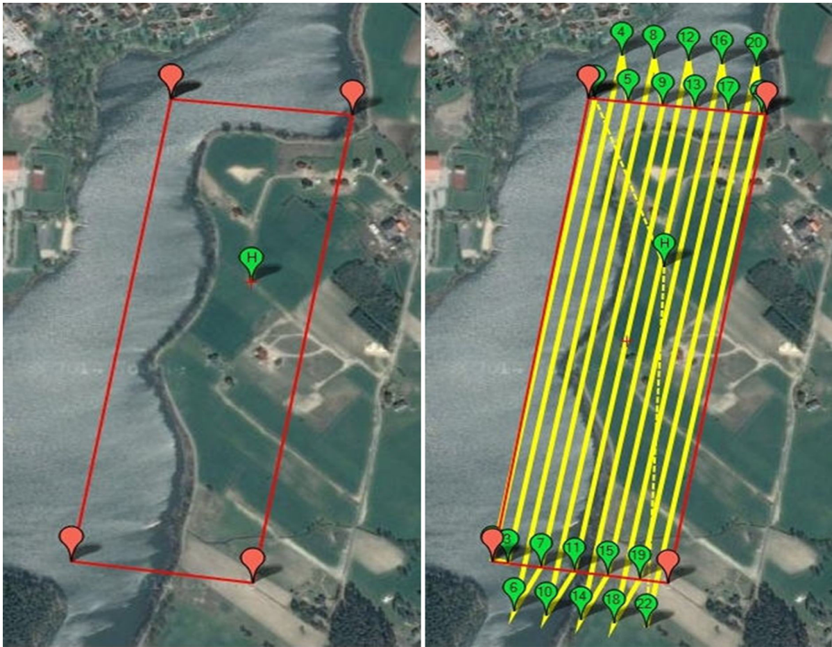
Figure 4 Investigated area (on the left). A flight path across the study area (on the right)
