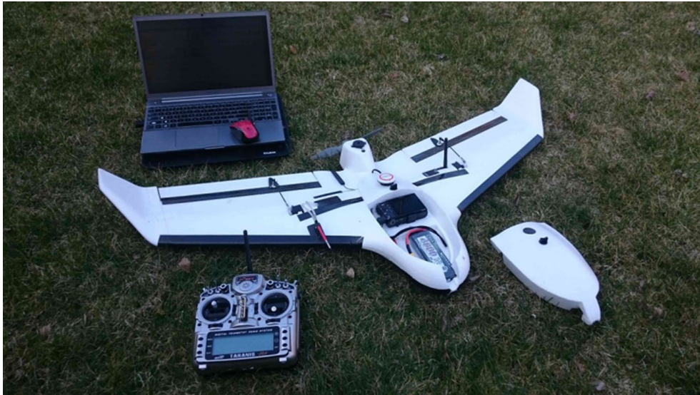
Figure 3 UAV system fitted with Sony RX100 camera
