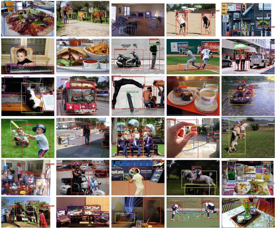
Fig. 5. Detection examples on COCO test-dev with SSD512 model. We show detections with scores higher than 0.6. Each color corresponds to an object category.
