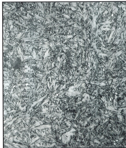
Fig. 7 Core microstructures of the 3" diameter bars of (a) 4340 steel and (b) 01 tool steel.
