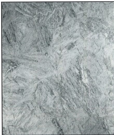
Fig. 7 Core microstructures of the 3" diameter bars of (a) 4340 steel and (b) 01 tool steel.
