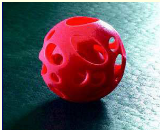
Fig. 2 This complex sculptural object was created using 3D modeling software, and then directly fabricated using a ZCorp 3D Printer.
