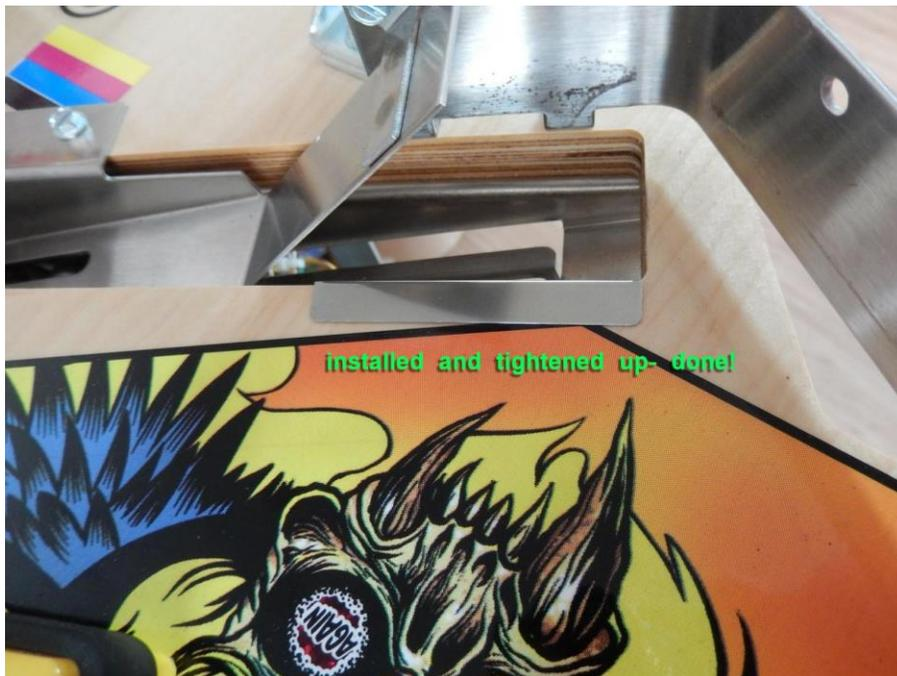
Trough screws tightened back up, done! Reinstall apron to complete
