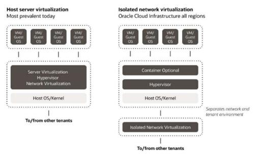
Off-box network virtualization enables running bare metal instances side by side with any class of systems—including VMs, containers, and optimized database systems such as Oracle Exadata—all using the same set of APIs. With Oracle Cloud, customers can leverage unique Exadata capabilities (including tens of millions of IOPS, I/O prioritization, and columnar compression) to run Oracle databases with cloud native security and advanced governance capabilities.
