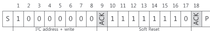
Figure 13: Soft Reset – grey blocks are controlled by EEH210.
