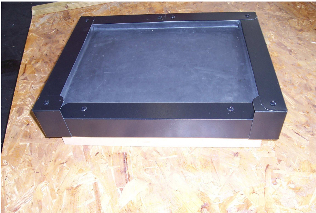
Illustration of roof model with trim detail; note radius formed on corners with sharp tin snips for neatness
