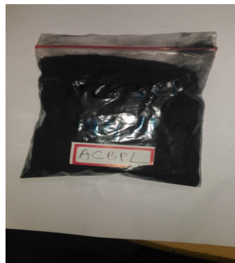
Fig.1: Activated carbons prepared from Bauhinia Purpurea leaves with average particlesize of 149 \mu\text{m} .
