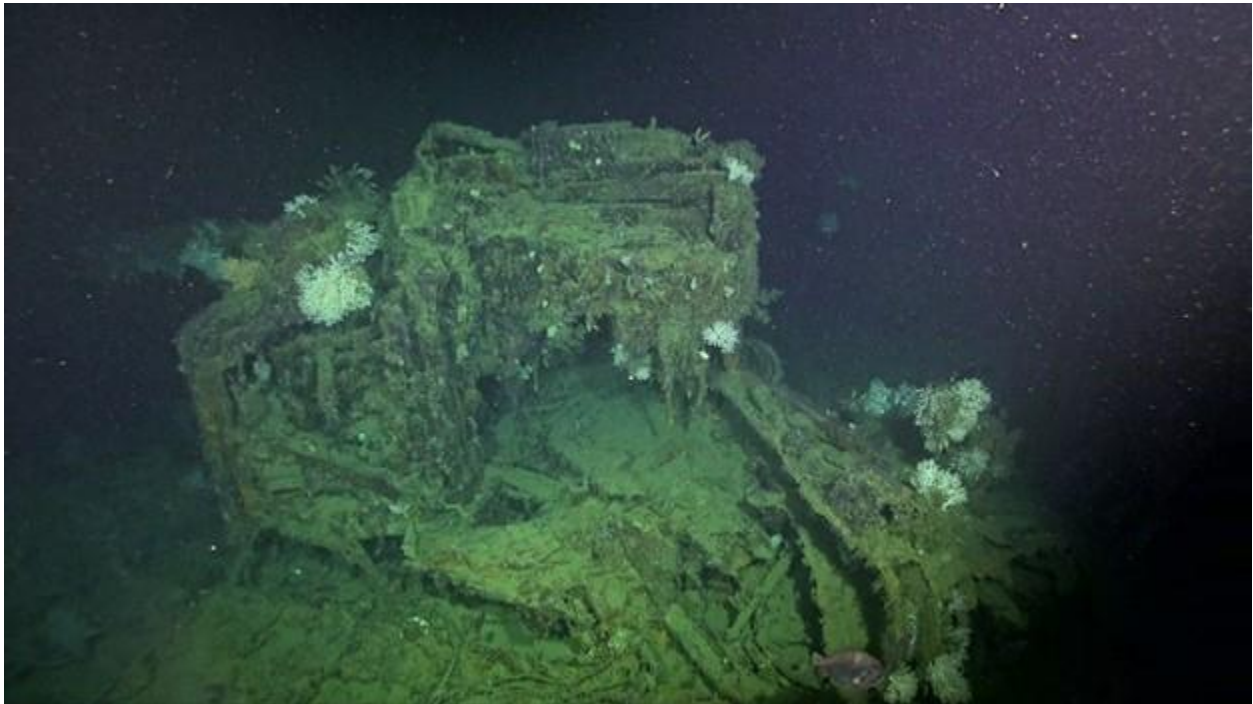
Figure 10 - The No. 1 gun mount on Monssen was struck by a medium cal. from port on top of No. 1 gun shield killing gun crew. This damage likely came from Hiei's secondary battery. Copyrighted by Lone Wolf Media.
