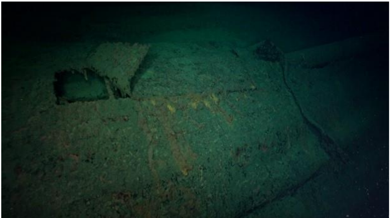
Figure 33 - This is Hiei's starboard outboard shaft which I believe shows shock damage from U.S.S. Enterprise's torpedo. Copyrighted by Lone Wolf Media.
