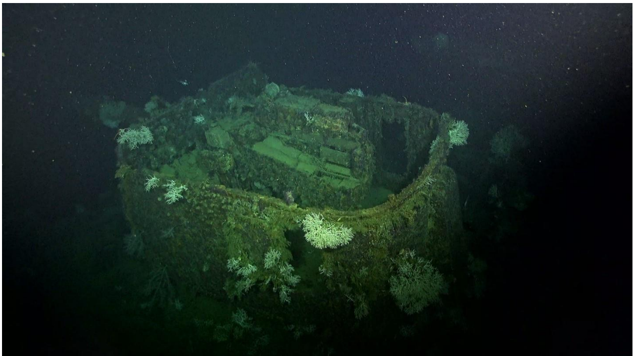
Figure 16 - Monssen's No. 3 gun pointing to starboard has lost its roof plate. Copyrighted by Lone Wolf Media.
