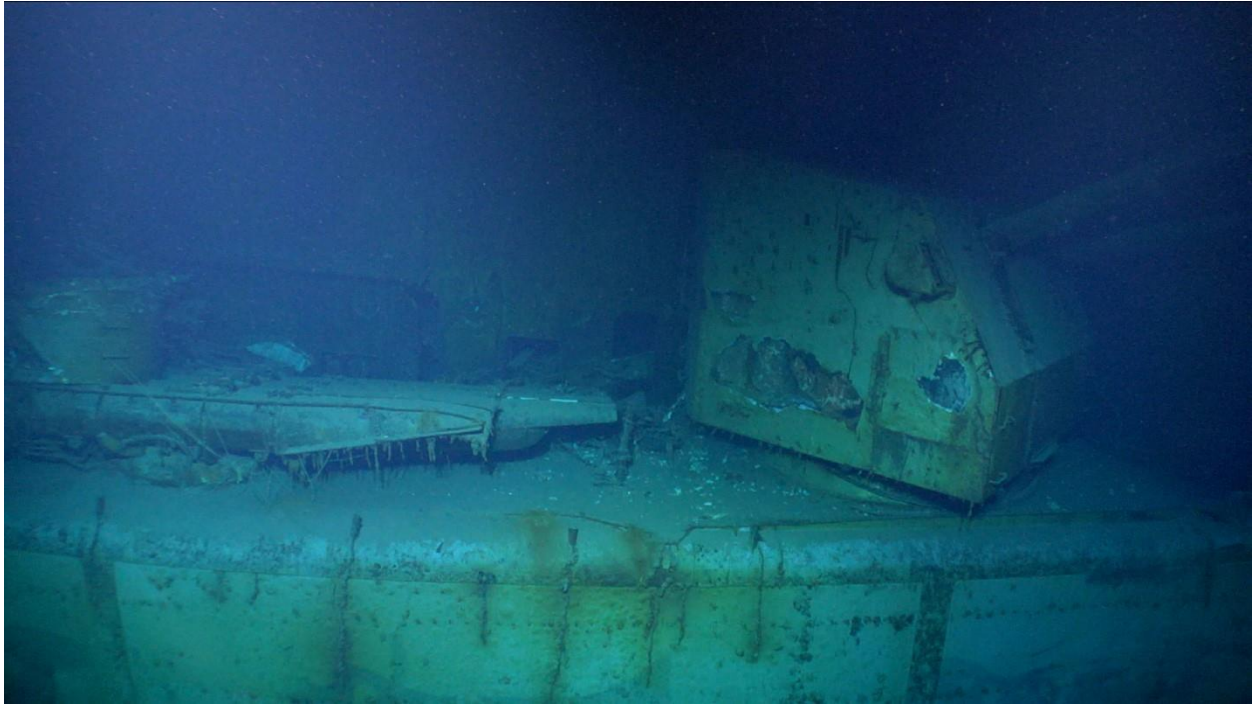
Figure 26 - Juneau's port side torpedoes still loaded and mount 55. Copyrighted by Lone Wolf Media.
