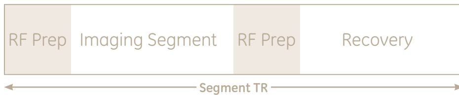
Figure 1. Pulse sequence timing for a 3D COSMIC acquisition. The RF prep and RF post segments improve the oscillatory signal state while the recovery period aids SNR by allowing recovery of the longitudinal magnetization.
