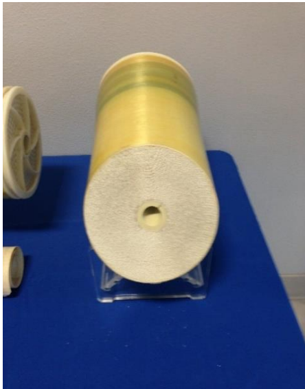
Figure 27 – The membrane in the trains through which feed water passes (Photo Credit: William Delgado-Thompson)
