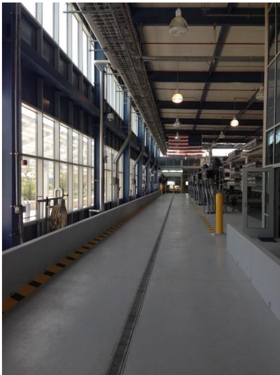
Figure 35 – Natural light plays a key part in illuminating the KBH plant (Photo Credit: William Delgado-Thompson)
