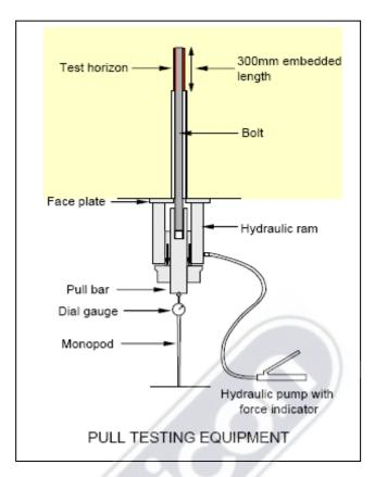
As per DGMS Guidelines, it is advised to carry out Short encapsulation pull testing of every batch of resin capsule. (Ref: DGMS/S&T/Tech Cir (approval) No 10 of 13th July 2009 & DGMS/S&T/Tech. Cir (Approval) No. -03 of 22<sup>th</sup> September 2010)
