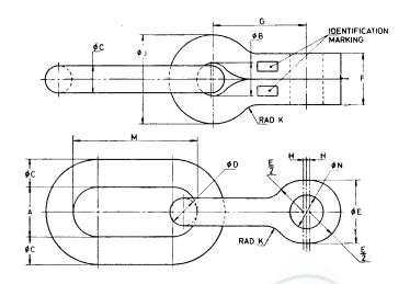
The design & specification of the Link and closed Shackles shall confirm to the drawing & specification as per as per DGMS (Tech) Circular No 7 of 1978 and as per IS 12488-1988. The use of Link and closed Shackles will:
