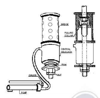
DGMS Circular No.19 of 1974 has advised that mines adopting roof bolting should be equipped with reliable and tested equipment for carrying out the Torque Test, Anchorage Test and Sag Test.
