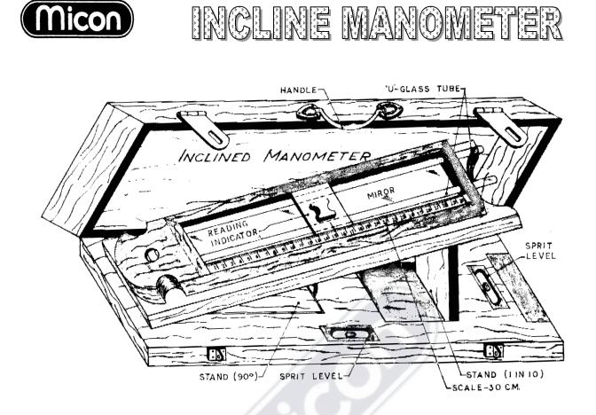
'Micon' Incline Manometer (water gauge) is used for measurement of small pressure with great accuracy. It consists of a 'U' glass tube of uniform bore filled with coloured liquid. U-tube is mounted on a wooden frame with Scale. The Frame can be locked in two positions.
