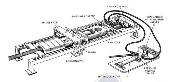
Micon Banding Machines are portable and provide the recommended alternative to the use of hammers and swages when capping wedge type rope cappels. The machines may be utilised for banding and disbanding all types and sizes of rope cappels.
