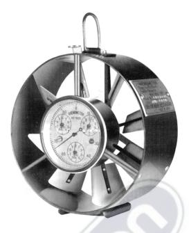
ANEMOMETER consists of a small fan or air turbine set at an angle of 40  $^{\circ}$  to 45  $^{\circ}$  to the direction of Air Flow which rotates the vanes at a speed proportional to the air velocity. The shaft or spindle actuate, through gearing, a series of pointers on the dial face of the meter, so indicating the distance in meters travelled by air in a given time. A clutch is fitted to enable the dial pointers to be put in or out of gear as required.
