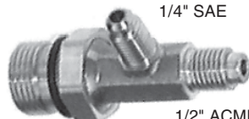
8720 Vacuum Pump Fitting - Retro-Adapter to convert R12 pumps to R134a
