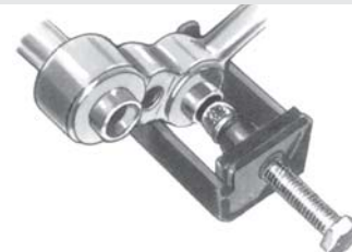
Special insertion tool seats the screen securely in the suction side
