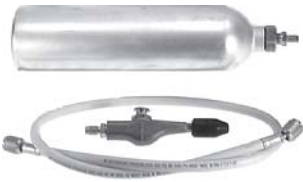
8805 - System Flush Kit Includes flush gun, hose, canister, and canister adapter. Uses shop air to propel flush solvent through each component.
