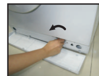
Unscrew the pump cover
