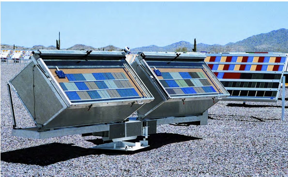
These AIM Boxes are used to test materials for automotive interiors. They offer single-axis sun tracking and can hold large, 3D parts like instrument panels. ( http://www.q-lab.com/test-services/arizona.aspx )
