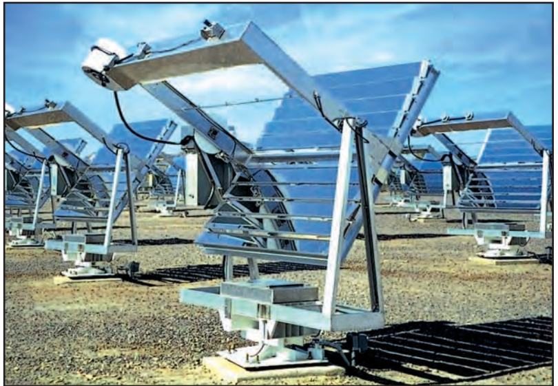
Q-Trac Natural Sunlight Concentrators at Q-Lab Arizona give realistic test results in less time than natural exposures. They change position throughout the day to follow the sun.
