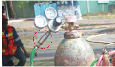
Fixed gas tank chain and installed anti-liquefaction equipment
