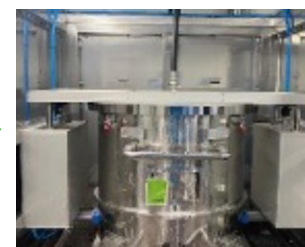
▶ Operating sealed hopper washing equipment and recycling system at Cheongju Plant
