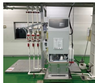
▶ Establishing TOC continuous measurement system at Cheongju/TP plant
