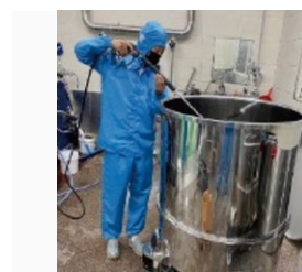
▶ Operating sealed hopper washing equipment and recycling system at Cheongju Plant
