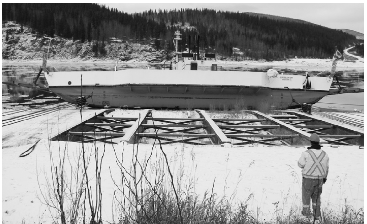
The boat spends the winter on this special pad, with cramped space underneath for workers to do hull maintenance in the spring.
