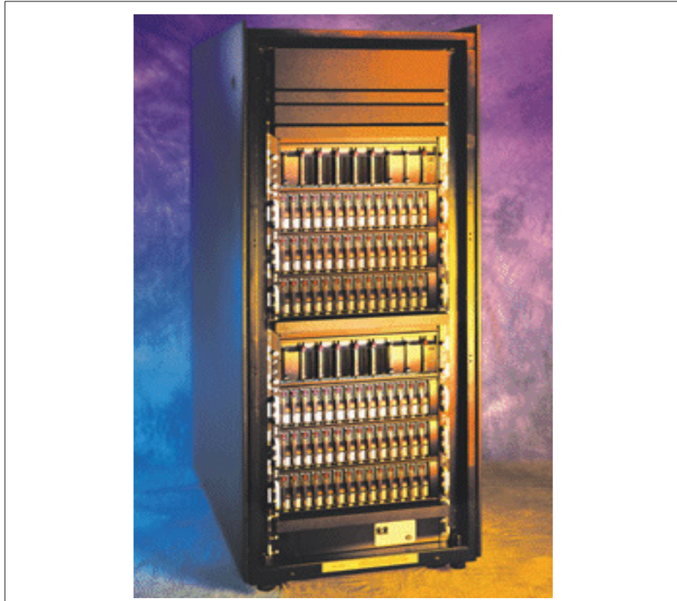
Figure 60. IBM Modular Storage Server
