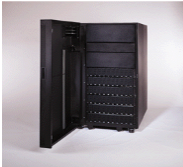
Figure 118. IBM Fibre Channel RAID Storage Server
