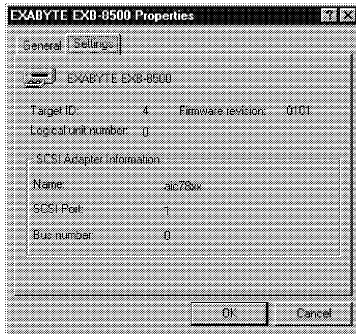
Figure 64. SCSI Channel Definition on Windows NT (4)
