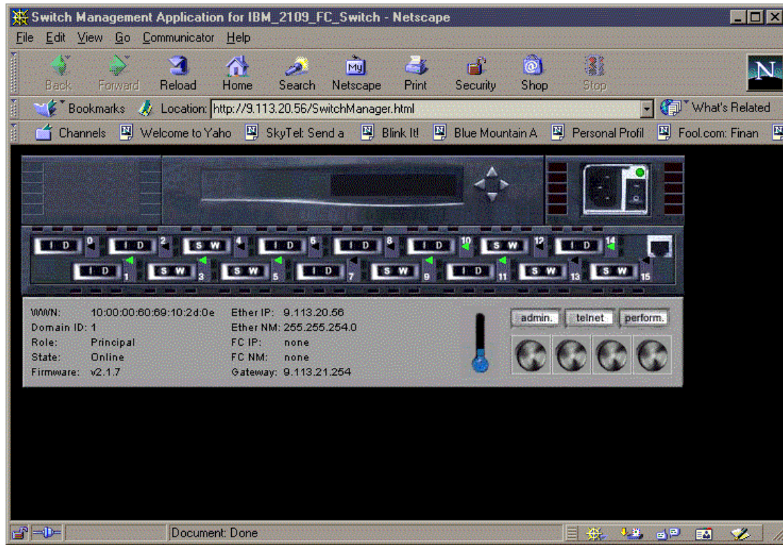
Figure 25. Brocade/IBM switch GUI
