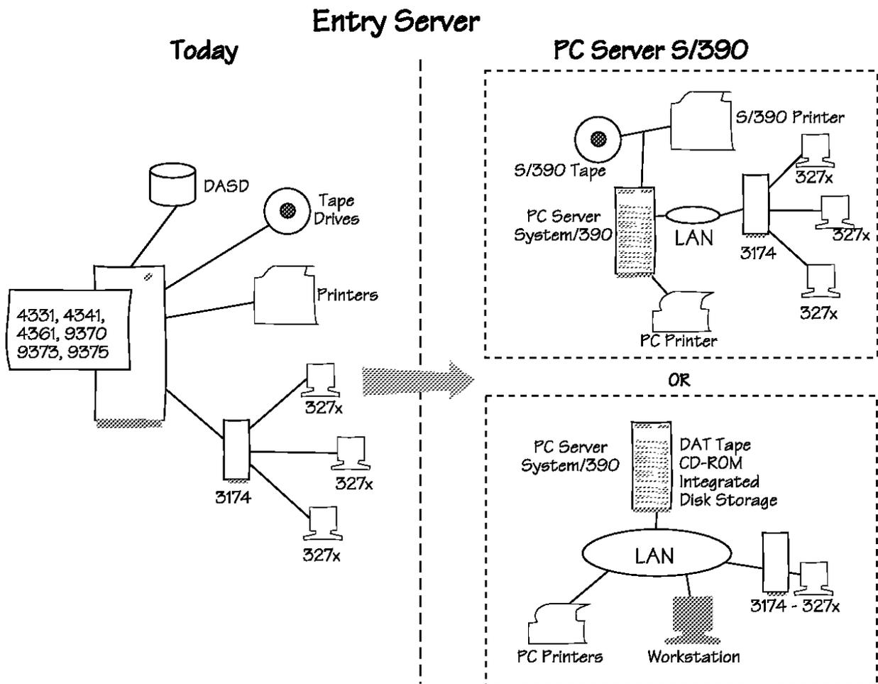
Figure 7. PC Server System/390 as an Entry Server
