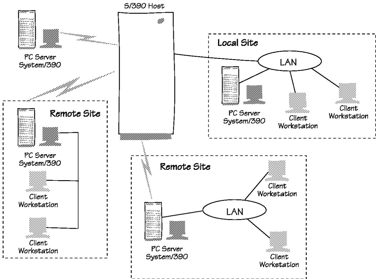
Figure 6. PC Server System/390 in Distributed Environments
