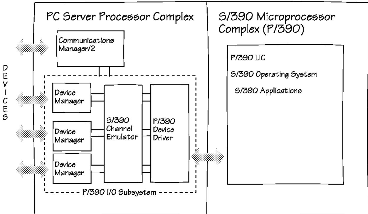
Figure 4. P/390 I/O Subsystem
