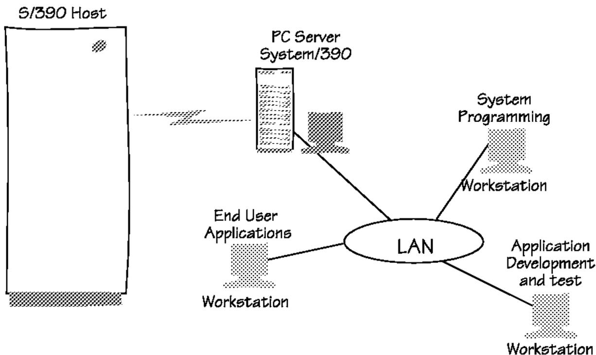
Figure 5. PC Server System/390 as a Development Workbench
