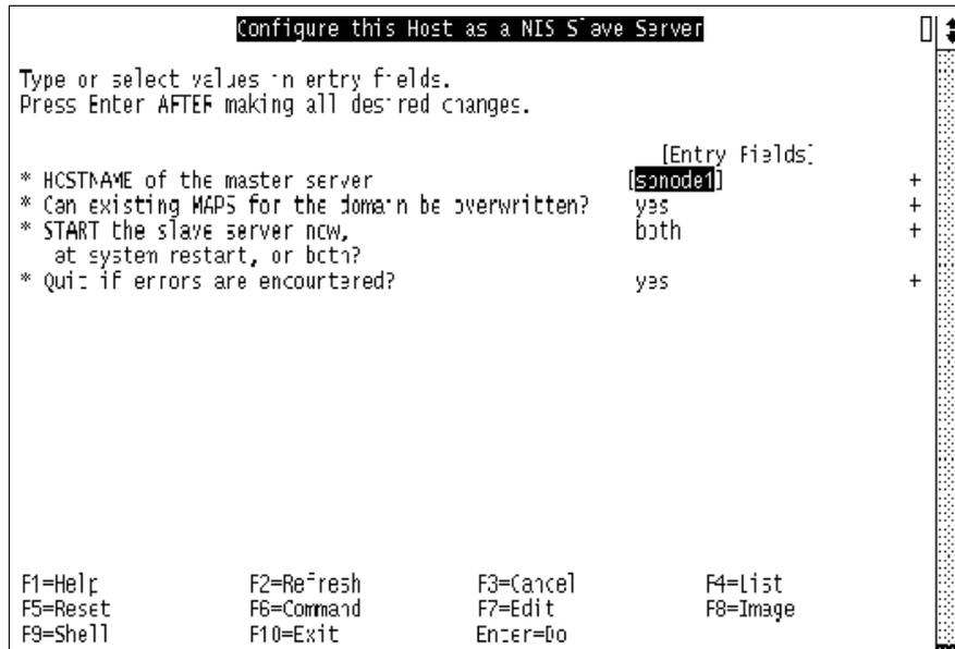
Figure B-3 SMIT panel for configuring a slave server
