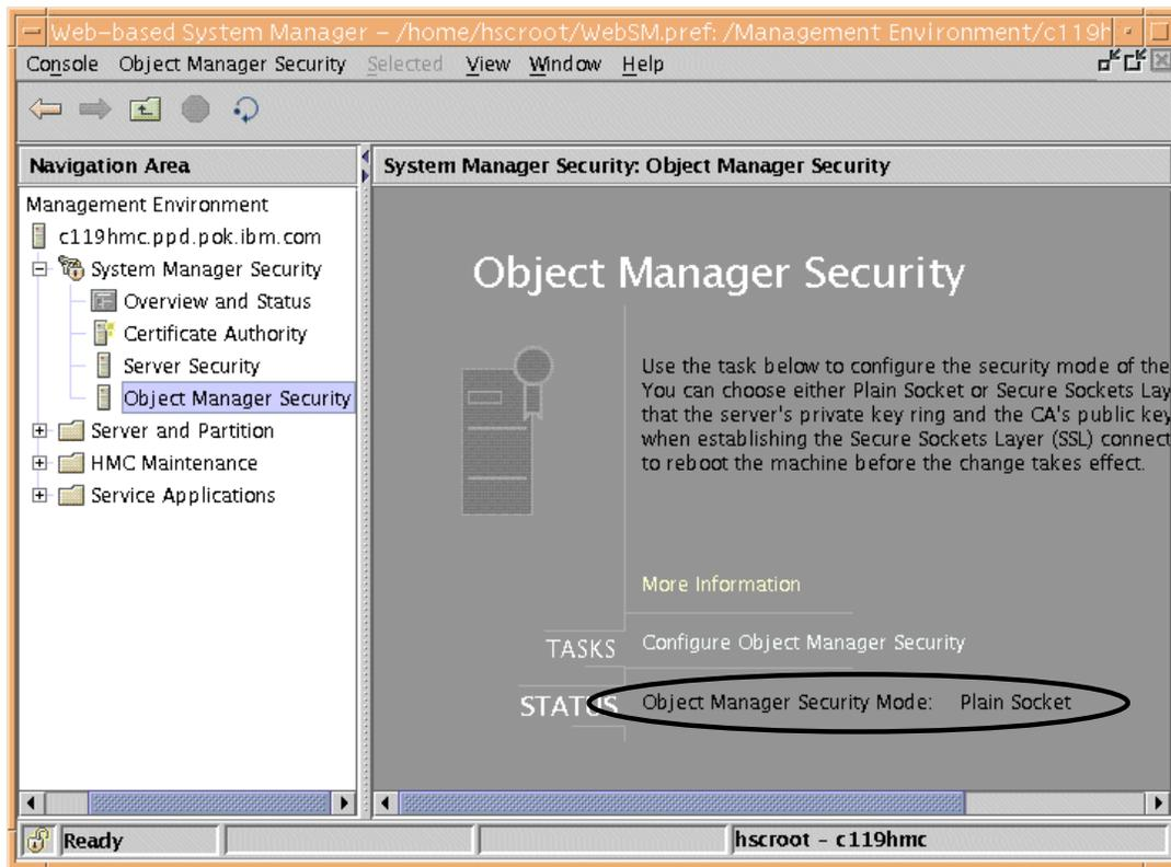
Figure 14-2 Setting the Object Manager Security
