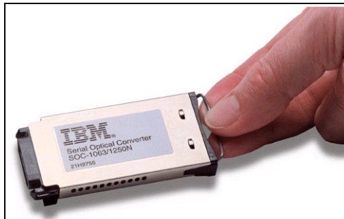
Figure 2-4 Gigabit Interface Converter
